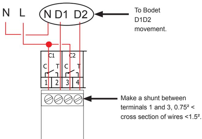
**⚠** Circuits must be protected by fuse disconnecter or circuit breaker 4A maximum. Indicate on the label above the terminal block the location of these protections.
