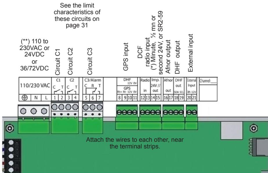
(\*) See page 25, the “Time outputs” menu to set this output (Pulse minute, ½ minute, second 24V or power TBT 24VDC 1A).
