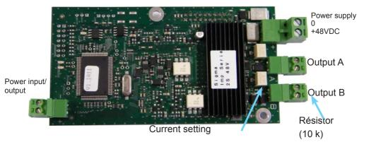
This option board does not require any programming. By default the time is the local time defined in the Sigma, with 1.2-second impulses, and the line is stopped.
