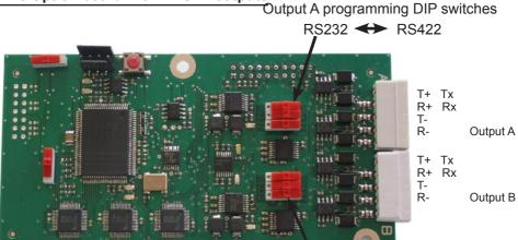
Output B programming DIP switches
