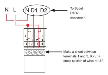
D1 D2 uses the relays of circuits 1 and 2
