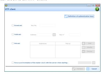
On this NTP Client screen, it is possible to choose the mode of transmission of the time signal.
