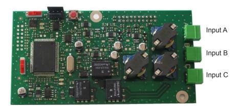
This card allows the addition of 3 external inputs.
