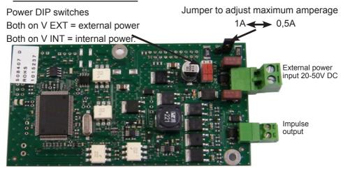
This option board does not require any software programming. It allows to add a minute, ½ minute, second or SR2-59 impulse output or TBT 24V DC 1A power supply. See page 36, the menu of the time outputs to set this output. Use the two Power DIP switches to select internal (24V) or external power (from 20 to 50 V).
