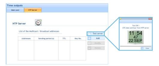
In NTP server mode, the Sigma sends the time to the selected IP addresses with the selected mode of transmission.
