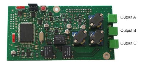
This option board does not require any software programming (by default the time is the local time defined in the Sigma and the line is stopped). Only the time zone differential and the state of the line (On / Off) is to be defined in the "Time outputs" technician menu (see page 36).
