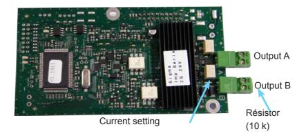
This option board does not require any programming. By default the time is the local time defined in the Sigma, with 1.2-second impulses, and the line is stopped.
