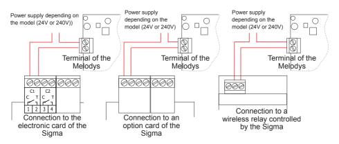
The Melodys can be connected directly to a relay output of the master clock, an option card or a wireless relay.
