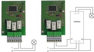
For relay circuits provide protection by disconnecting the fuse or circuit breaker maximum 4A. Please indicate on the terminal label the location of these protections.
